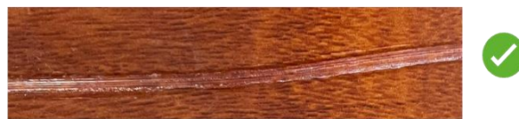
Cabling too fast, adhesive not fully melted
