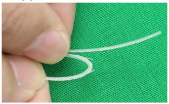
**Step 3** Cut off the extra sheath of the optical fiber and ensure that the end faces of the sheath on both sides are flush.
