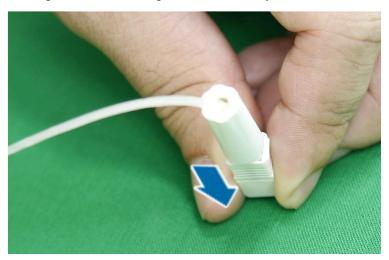
**Step 2** The lock of the connector body is exposed. Push the lock to the ON position.
